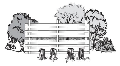
*Wildlife Observation Blind:* A simple structure with a solid wooden wall with slats cut out at eye level will allow students to view wildlife on the other side. It should be placed in front of bird feeders, wetlands, in meadows or along thickets for closer observation of secretive wildlife. See diagram for basic design.
